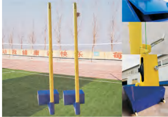
SC-88274 移动齿轮升降排球柱 Move the gear to lift the volleyball post 箱体40cmx60cmx30cm可加砂石水泥配重 ,立柱外管是89cm内管76cm,壁厚2.5mm调节高度2.24米-2.43米 QTY: 1set=3pkgs (底座2件+立柱1件) G.W:70kgs/set (配好重量250kgs左右) MEAS:105x60x30cm (底座x2件) 190x23x13cm (立柱) 建议零售价: ¥4500/set
